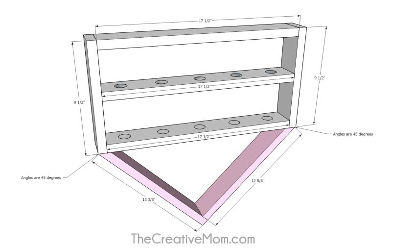
Cut 1- 9 1/2" 1x3- Both ends are cut at 45 degrees. Measurement is taken from long point to long point.
