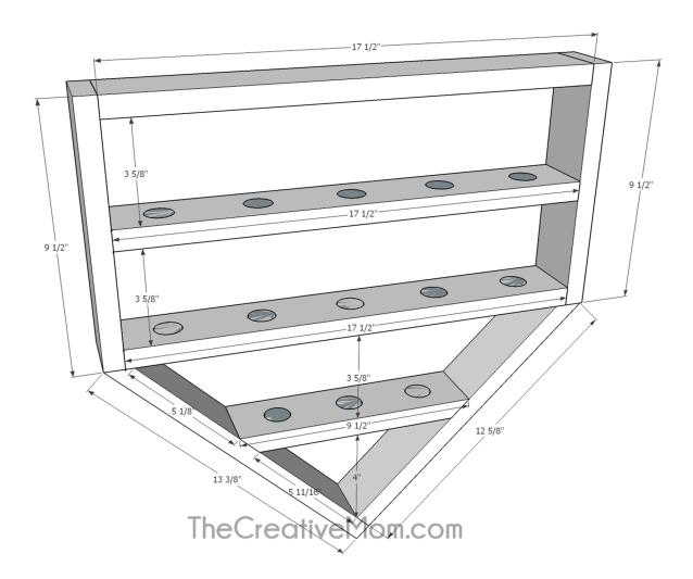
Optional: Lay your shelf onto a piece of 1/4" plywood and trace around the edge. Use a miter saw to cut. Attach the backing with wood glue and brad nails.
